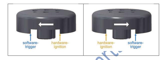
If the particular edge of trigger-window passes the center of magnet in the stator, the appropriate action occurs. Here is an example for clockwise rotation.
