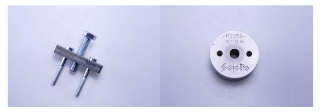
Screw in the screws completely so that the forces cannot tear out the thread.
